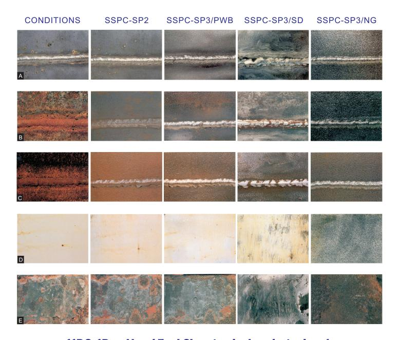
\$\$PC-\$P2 Hand Tool Cleaning by hand wire brush
