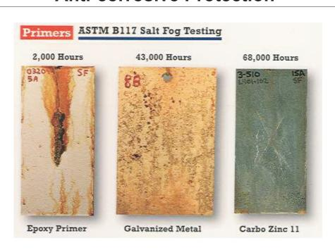
When properly applied and maintained, there should never be a need to remove a zinc rich primer on a water tank. Based upon a 100 year life span, and proper overcoats with Peacofour 6700, the tank's old coatings should never have to be removed (Other high-performance primers are also available for use with Peacofour 6700.)
